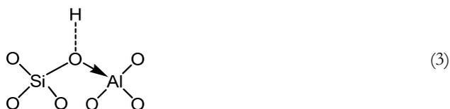
Upon severe heat treatment (> 500 °C) the Brönsted acid sites are removed (dehydroxylation) and water is split off with the concomitant formation of Lewis acid sites. The precise chemical nature of Lewis acid sites is less clear. They can be looked upon as tricoordinated aluminum and/or tricoordinated, positively charged Si in the framework<sup>26</sup>.
