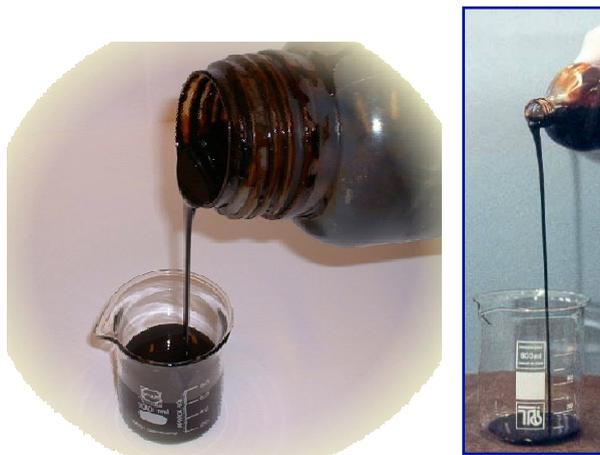
Figure 8 - Bio oil produced by lignocellulose pyrolysis, Bio-Oils composition: Water: 20-30 % C: 44-47 %; H: 6-7 %; O: 46-48 % N: 0,2 % max; S < 0,01 % density 1,2 Conradson Carbon : 10 - 20 %.
